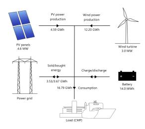
**Figure 6.2:** Overview of the system with the highest utilization for the shore power scenario (Scenario 8.0.5). Energy flows and capacity are presented with arrows representing energy flow directions.
