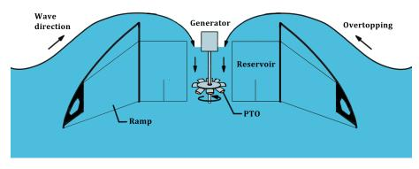
Figure 2.20: Basic principle of OWAEC technology.
