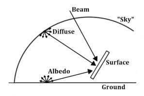
Figure 2.3: The three different components of solar radiation.
