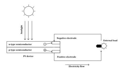
Figure 2.1: Typical PV cell technology.
