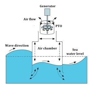
Figure 2.19: Basic principle of OWCWAEC technology.
