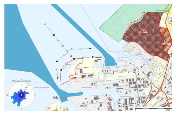
Figure 4.1: Some possible siting layouts for 3 MW wind turbines. Hatch marks nature protection areas. Red outline marks the proposed expansion of the harbor. Darker blue is sea lanes. Distances given in meters or rotor diameters, D=112 m. The wind rose for Oskarsgrund is presented as well. Map taken from [39].
