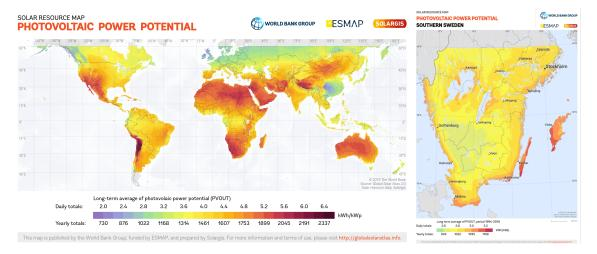
Figure 2.5: PV power potential in the world and specifically southern Sweden. The text in the figure is not relevant, of note is that red areas have more irradiation whilst green and blue areas have less irradiation. Image taken from [8].
