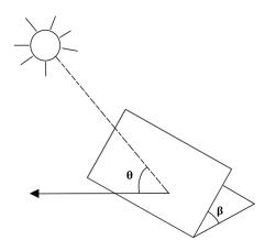
Figure 3.6: Definition angle of incidence
