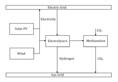
Figure 2.28: The principle of power-to-gas.
