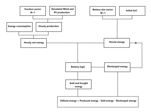
Figure 3.7: An overview of the optimization process. This diagram represents the optimization of PV, wind and battery presented in Section 3.5.3. For the PV and wind optimization the hourly net energy is directly used to calculate the sold and bought energy (discharged energy is not used).
