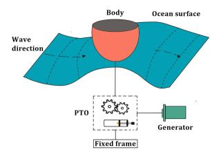
Figure 2.18: Basic principle of OBWAEC technology.
