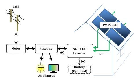
Figure 2.2: Typical grid-tied PV system.
