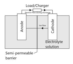
Figure 2.23: Schematic drawing of a battery.
